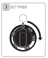
The timer is the main ON/OFF switch. Turn the dial to the required amount of time. The red light will illuminate when the timer is running.
